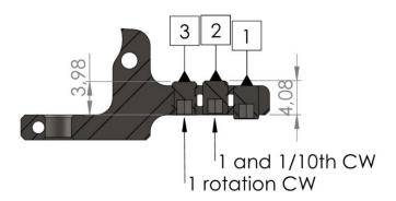
C Stage adjuster combination screw 1 & 3 (solid weight release/Hunting/Plinking)
