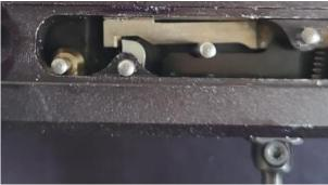
**Step 4:** Choose either the 10 or 15mm 1<sup>st</sup> stage spring and slide it over the small tab of the adjustement screw. Now screw it into the triggerbase making sure the spring seats well in the triggersear spring recess.
