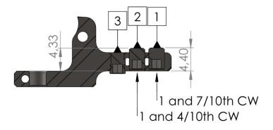
**B\*** Stage adjuster combination **screw 2 & 3** (middle weight release/Match/PRS/Hunting)
