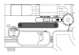
**Step 5:** Take out the dowel pins marked with the arrows, using needle nose pliers. Take care not do damage the pins
