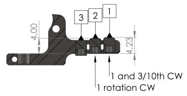
**B\*** Stage adjuster combination **screw 2 & 3** (middle weight release/Match/PRS/Hunting)
