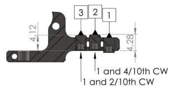
C Stage adjuster combination screw 1 & 3 (solid weight release/Hunting/Plinking)
