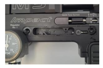
**Step 1:** Take the triggersear and the triggerbase and remove the spring adjustment screw of the 1<sup>st</sup> stage so there is no tension on the parts. Apply a little grease (ballbearing grease for instance) on the contact area's where both parts interact with eachother.
