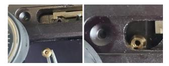
Line the part up with the dowel-pin holes. Push the dowel pin in with the chamfered side down the hole. Carefully push the dowel pin down until it is fully seated.
