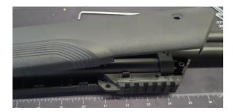
Remove the front screw from the picatinny rail that connects it to the barrel band.
