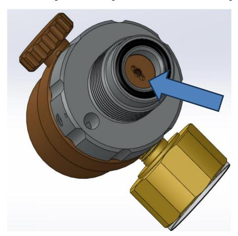
With this screw you can set the maximum outgoing pressure. Screw the stainless steel part of regulator directly into the valve of the scuba bottle, (If you use an external fill set, it can be screwed into the regulator female DIN 300 connection)
