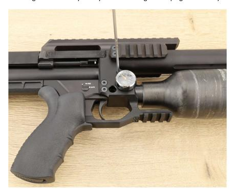
After you don't hear any air escaping anymore check the gauges for risidual air and dryfore it one tp make absolutely sure you have no air in it.
