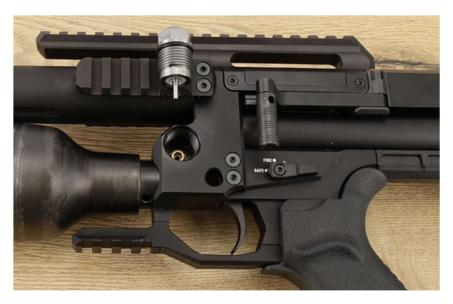
Using a 4mm hex key unscrew this brass plug. You'll find an o-ring underneath it. This oring also needs to be removed
