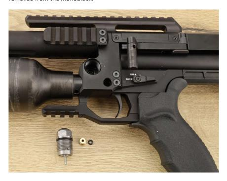
Take the parts from the package and unscrew the piston subassembly from the black regulator body, for assembly you will only need one valvedisc. Extra are supplied in case one might not seal properly
