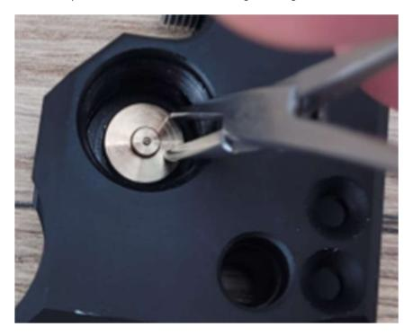
Now insert one of the valvediscs (just one) in the black regulator body it should stay in place by the silicone grease that is in the regulator. Note 2 valvediscs are supplied. The 2<sup>nd</sup> one is a spare in case the first one does not close accurately and you experience some creep on the oring!
