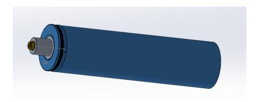
Use some silicone grease to "glue" in the face sealing oring
