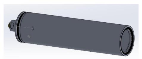
Now screw in the extension tube+valvehousing on the air tube. Leave a small space between the extension tube and the airtube to get a path for the atmospheric pressure to reach the regulator (a papers width will suffice). The whole assembly will look like this
