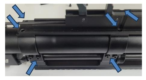
Before sliding of the clamp/toprail subassembly you will need to measure it's distance relative to the breechblock. In our case this was  $\pm 19$ mm
