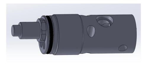
Now screw in the valve body in to the supplied cylinder extension. Before you do so apply some pure silicone grease to the orings.
