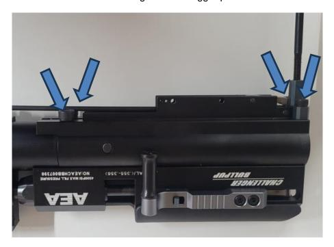
Now you can remove the complete trigger assembly and breechblock/barrel from the tube
