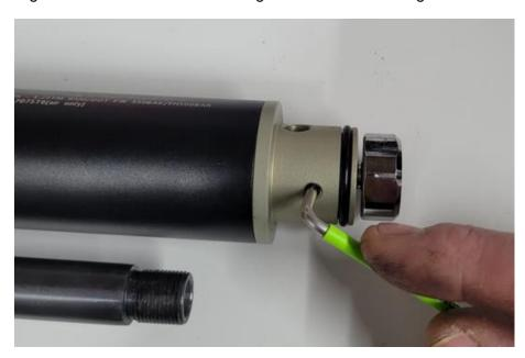
Unscrew the shroud from the gun and remove the centering ring from the front of the barrel
