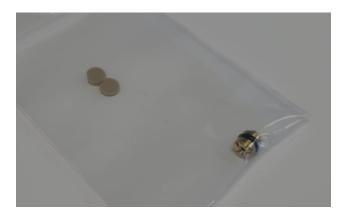
The discs has one sharp side and one side with rounded edges. The side with the rounded edges should face the nozzle and the side with the sharp edge should rest on the piston.
