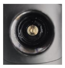
Now it's time to screw the locknut to secure the nozzle securely. Start using your fingers, Once you feel oring resistence switch over to a coin. €0,05 fits nicely. Use a coin that is less than 22mm Ø. And less than 2mm wide. The slot is 2.2mm wide. We do however offer a Raptor tool that is a perfect fit and we recommend using that!
