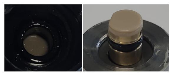
Then insert the piston subassembly in the locknut and screw it down until you feel resistence! Do not force the subassembly as this may damage the valvedisc. The other side of the raptor tool has the fitting hex connection.
