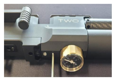
Make sure that all air is drained by checking the gauge first and then try and dryfire the Epic 2 to make sure it is completely empty.
