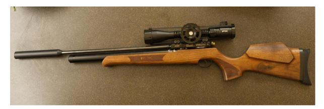
Best to remove the action from the stock. It isn't completely necessary but it will give you access to all the parts better
