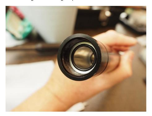
Now screw in the valvehousing not completely tight but leave a small gap the thickness of a piece of paper so the regulator can breath
