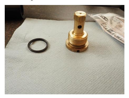
Grease up the regulator and insert it into the tube in the direction shown
