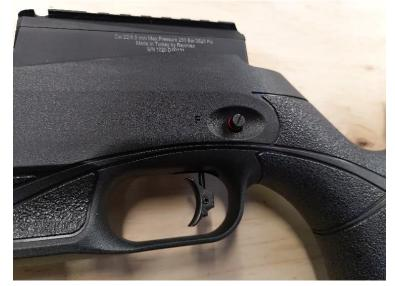
Remove the stock by undoing the screw on the underside with a Allen key.
