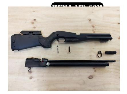
The action and aircylinder can now be seperated from the stock.
