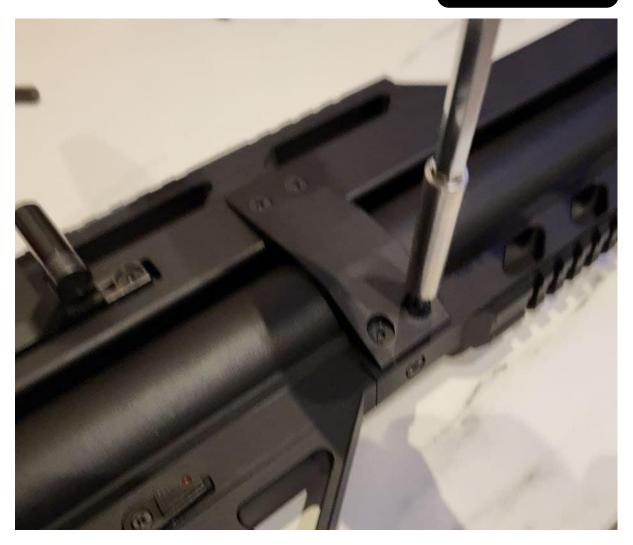
You need not to actually remove these screws, just loosen them until you can slide the tube from the action.
