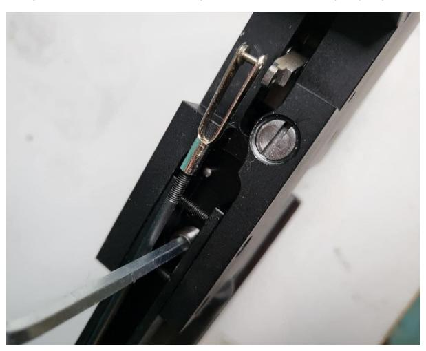
You could also remove the trigger linkage that goes back to the action and actuates the shear to make it easier to access this set screw, to do that just spread the two legs so the linkage can slide out of the captive hole as indicated below.
