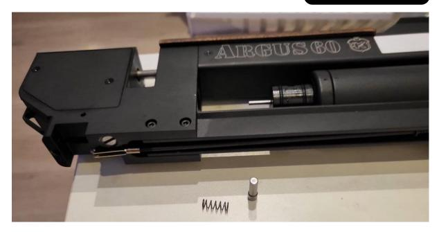
Now continue working on the cylinder. We need to unscrew the valve body from the cylinder. This could be a bit stiff and hard to unscrew. If it is, and it'll probably be the case, stick an allen key or something similar into the transfer port and gently use it to get more leverage to unscrew the valve body as shown below.
