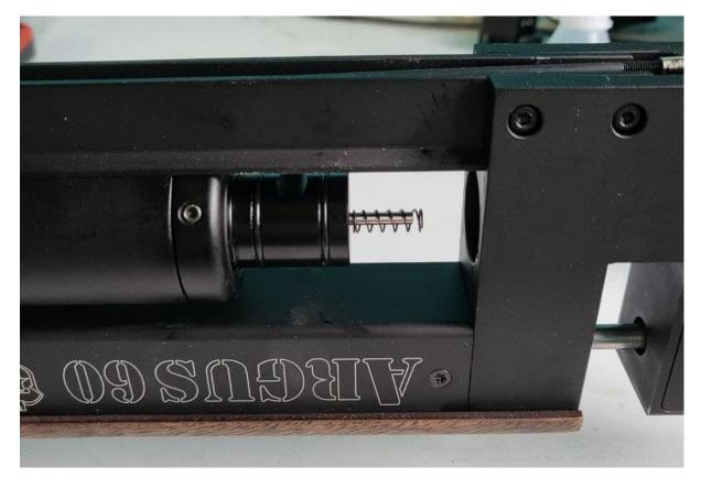
Now tighten the large setscrew and tighten the 4 screws on each side. Do not over torque these screws.
