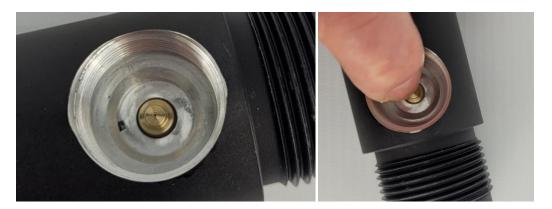
Now it's time to screw the locknut to secure the nozzle securely. Start using your fingers, Once you feel oring resistence switch over to a coin. €2 fits nicely. 10pence (GBP) or a Nickel, half a dollar or a dollar (USA) will also work well. Shipping cart coins will generally work well. The slot is 2.2mm wide.
