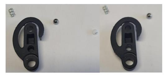
Now the spring and detent can be reinstalled. The ball will sit a little more prone of the face of the safety. And reinstall it in the subframe.
