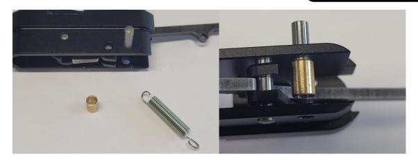
Install the spring as shown (this is reverse from what is generally the case in the Leshiy 2). And slide home the pin
