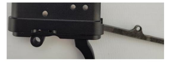
Take the small brass bushing from your kit and install it in the frame as pictured below. Partially slide the pin in like shown while keeping the bushing in place with a set of tweezers. Afterwards it looks as below.
