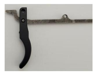
Now insert the Triggerblade and pushrod that you previously subassembled into the Trigger subframe from the top and insert the pins, after we will install the spring
