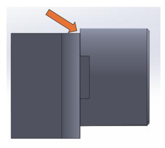
Above you can see the corner that will interfere with with the Backbone.
