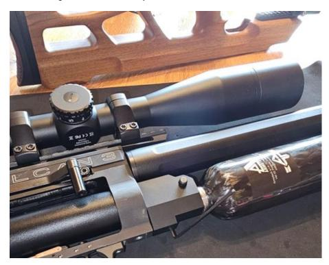
When the gun is completely empty you can unscrew the two locking screws that hold the plenum tube/valve/bottle subassembly in place. The screws are located on the underside of the rear action block, just in front of the trigger assembly. They will require a 4 and a 3mm allen key. You should be able to get past the trigger linkage, but you may wish to disconnect the clevis from the trigger parts, this can be done with a flat bladed screwdriver.
