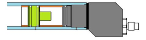
For the small plenum configuration insert the large plenum first than the regulator and then the small plenum.
