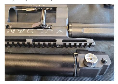
Next step is to unscrew both the front bottle block and the firing valve. This will help you to push out the OEM regulator.
